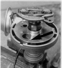
We used a single-point distributor for this conversion. If you have a dual-point setup, you'll need to use the supplied low-profile screw in the breaker point mounting hole closest to the where the wire exits (arrow). You'll also need to snip off the crossover wire as closely to the spade terminal as possible.
